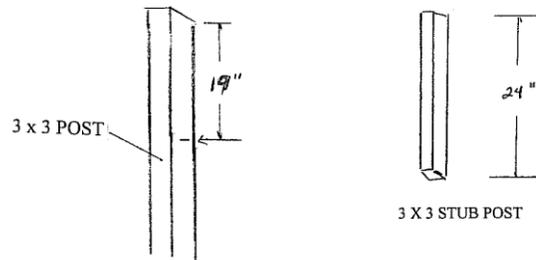
NOTE: If you are using double 2x6's for headers instead of the 3x8's, the mark should be 17 1/2" from the top.
