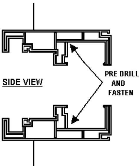
and fasten doorframe to mullions on all four sides with #8 x 1" tek screws. There are enough screws supplied to fasten four screws to each side of the doorframe. After securing the frame seal the holes.
