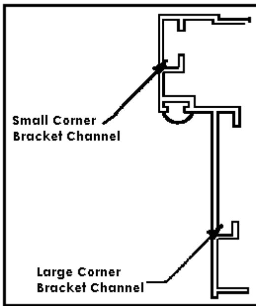
bracket a couple times and then the small bracket. Repeat the process until the corners of the frame are matched up.
