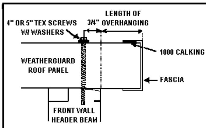
The roof will leak without additional sealing. To ensure a long dry life of the room, run a small bead of silicone (not polyurethane) on every seam.
