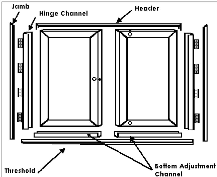
Assemble the Header and Jambs together by inserting the corner brackets of the Header into the channels of the Jambs shown in **Diagram 10.1**.
