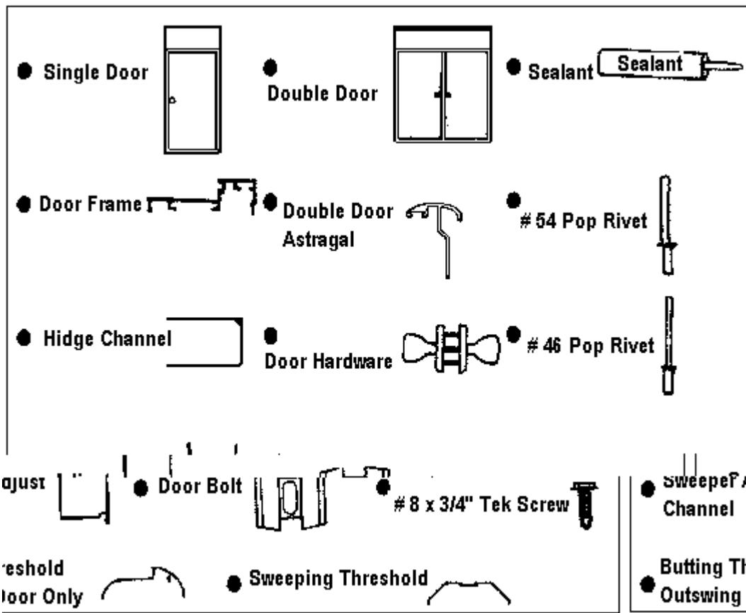
Unlike the Sliding Door, The Pedestrian Door is placed in the wall the same way a section is. Its sides are normally constructed with either a male or female mullion. The single frame is assembled while the double frame will require some assembly.
