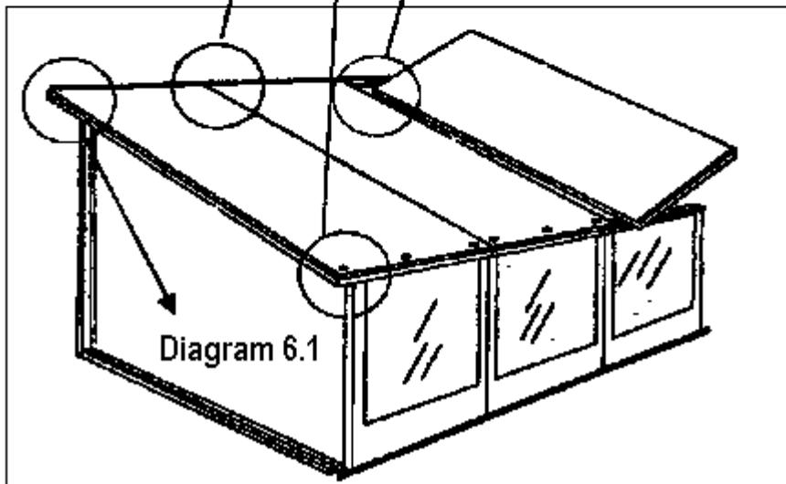
Channel and overhanging the Header Beam. Tilt the panel up and push towards first panel until the top of the panels are interlocked.
