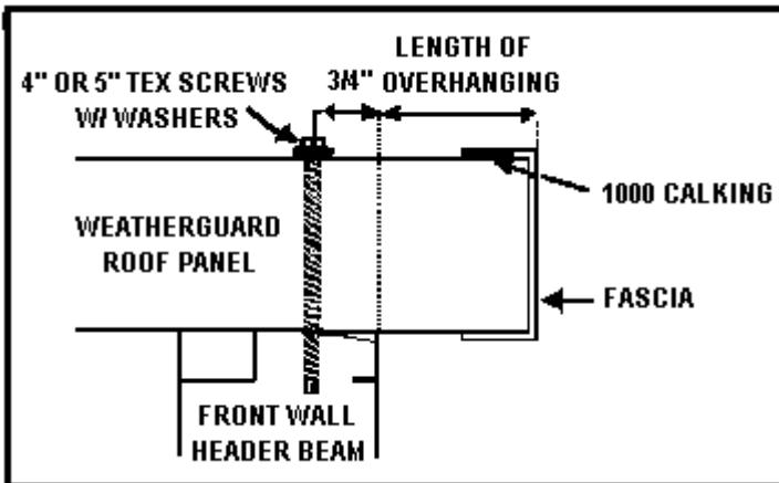
attached, (4" roof will require 5" lag screws) finish securing the roof panels with screws 12" on center.
